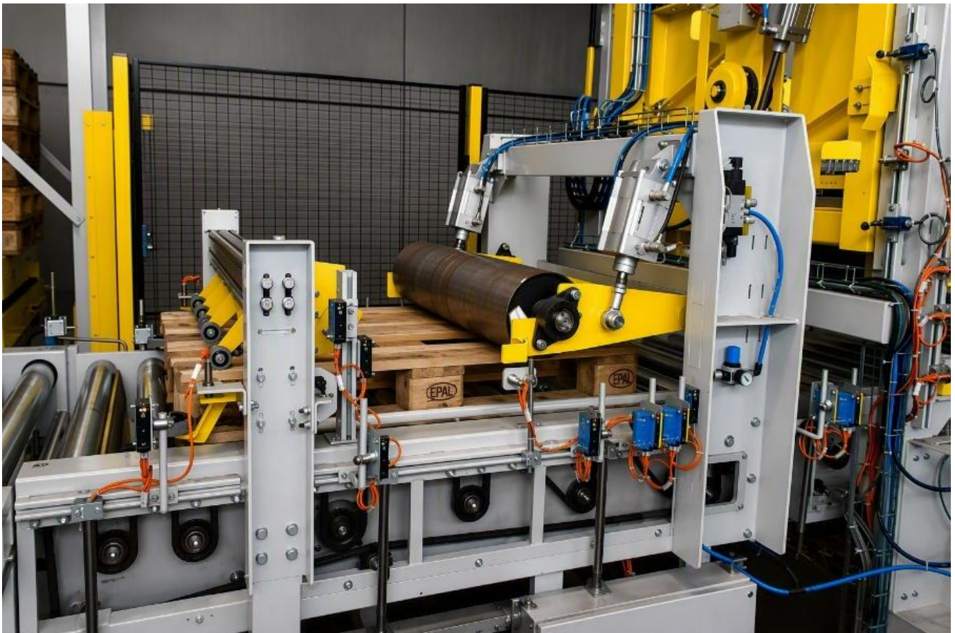
Motus Handling's Automatic pallet control and sorting system, one of the solution designed by Motus Handling to cope with damaged pallets.
